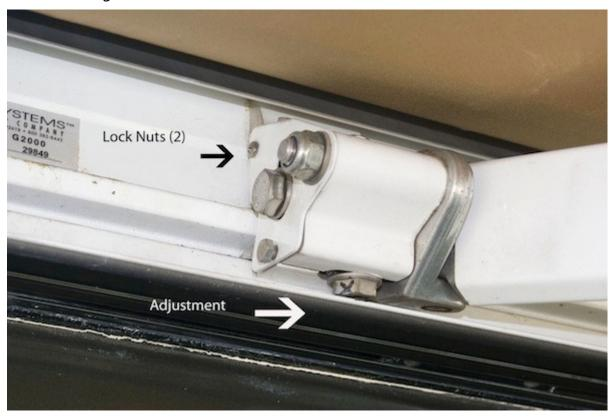
Tighten the fabric lengthwise. Put awning out almost all the way, stop 1 foot short. Start at rear. Remove the screw that holds the fabric to the outer rail. On ladder push the rail toward the MH and stretch the fabric toward the rear. It should move the fabric some. Release and replace the screw. Do the same thing at the front end of the awning. Figure 2.
