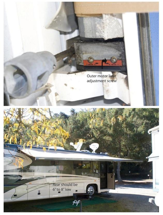
Do not over use the motor as it will overheat. So to check changes, only move it a short distance or wait between moves.
