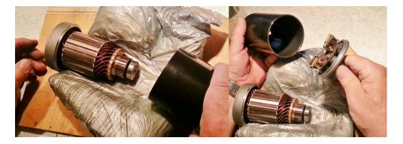
It is necessary to pull both end caps off to reassemble the brushes and commutator.
